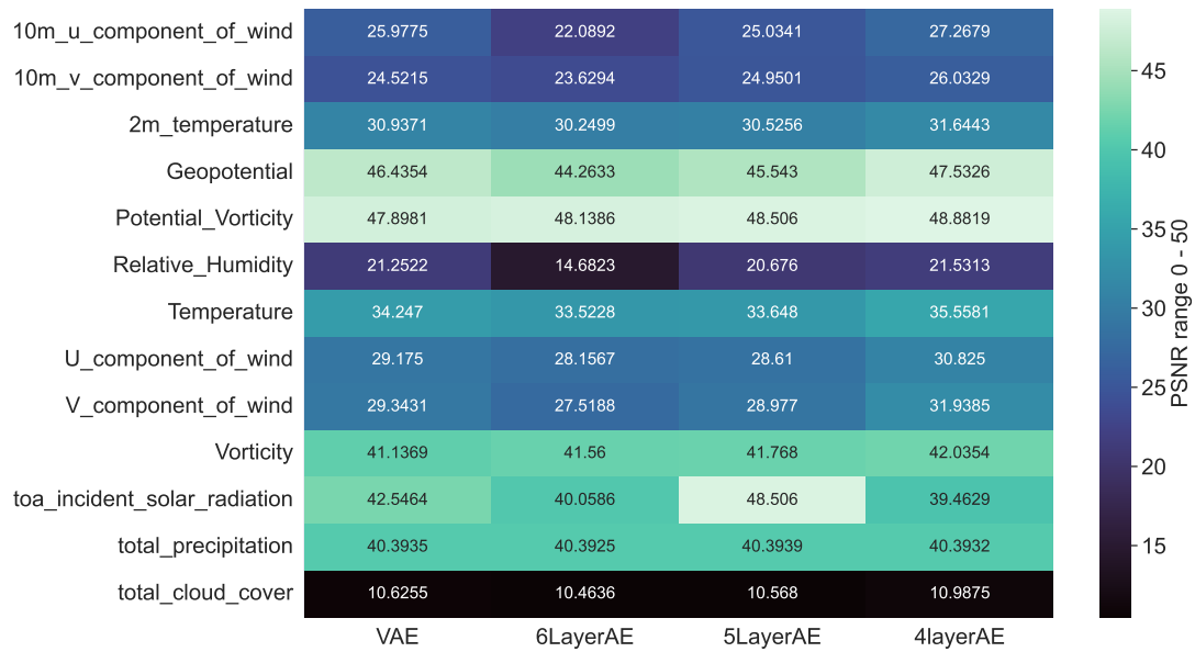
Figure 5.18.: Peak signal to noise ratio comparison of the variables across the implemented Autoencoders
